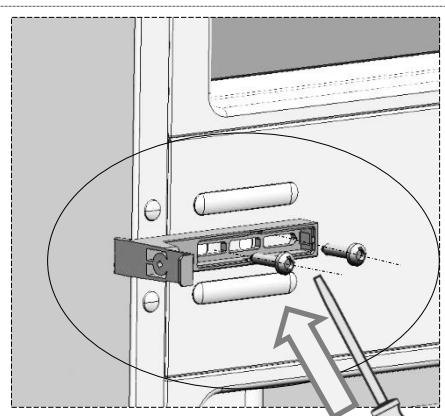
Installation step for 7: screws should not be fully tightened at this stage.
