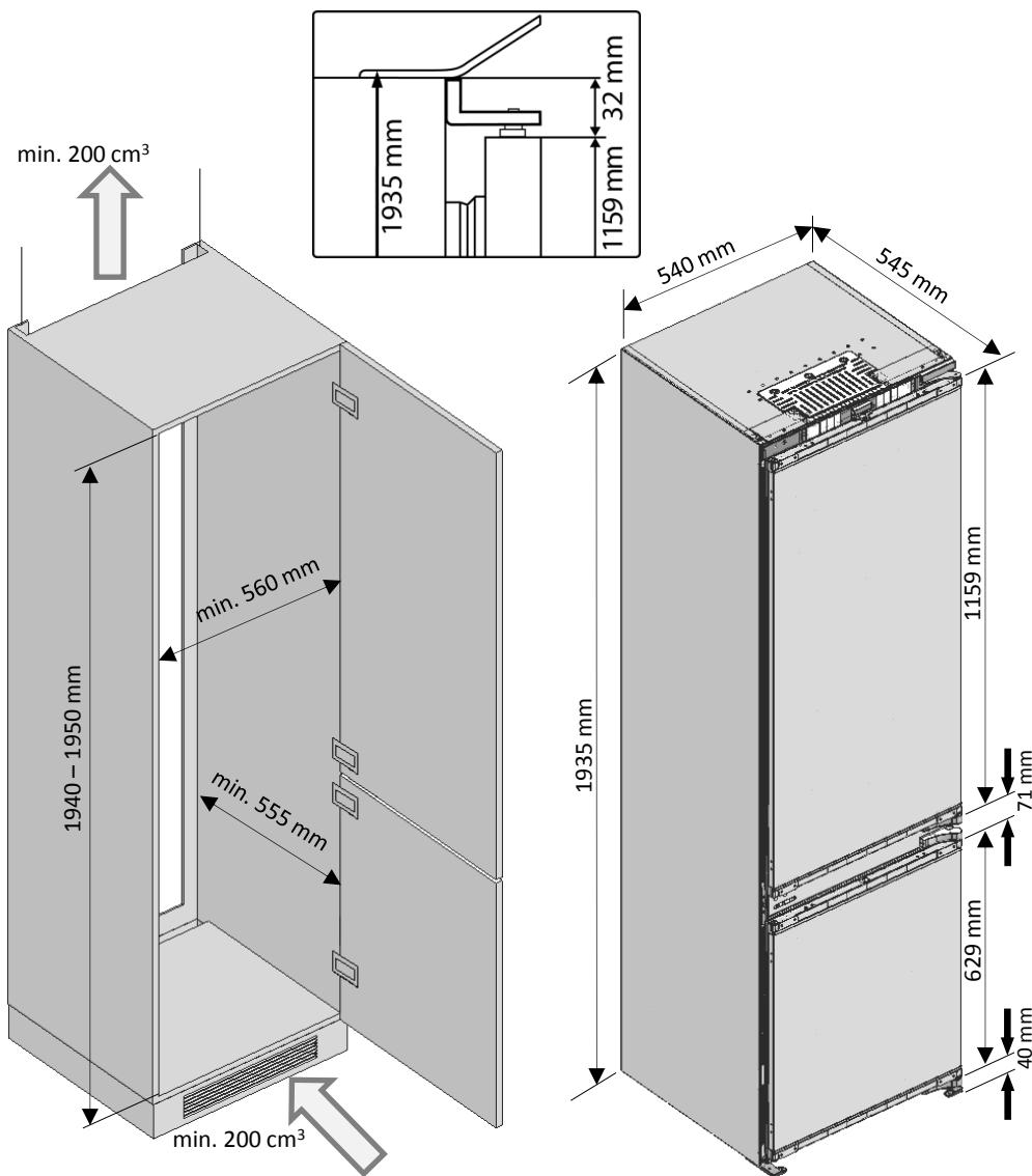
*The back wall of the wooden cabinet must be left open completely to kitchen wall in order to allow sufficient air circulation to cool down the condenser unit for energy efficiency.*
