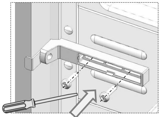
Installation step for 13: screws should not be fully tightened at this stage.
