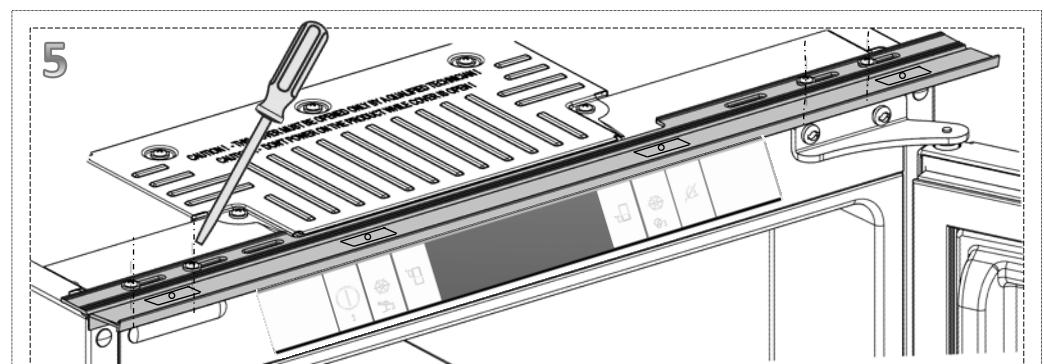
**Note:** screws for connecting top plastic part should not be screwed very hard, because of moving the plastic part easily left or right side.
