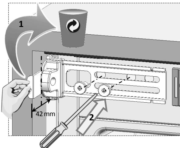
Installation step for 15: screws should not be fully tightened at this stage.
